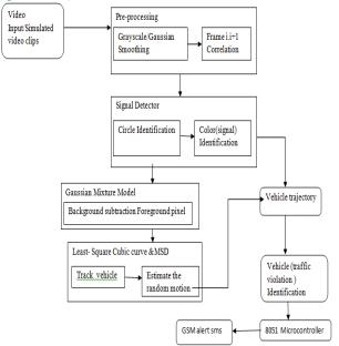
Figure 1: Block Diagram
