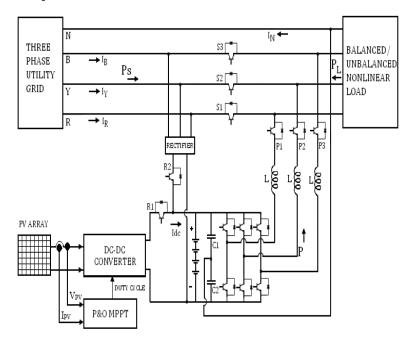
Figure 1: Schematic diagram of proposed PV-DSTATCO
