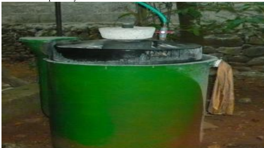
Figure 1: Photograph of Plastic Made Floating Dome Biogas Plant
