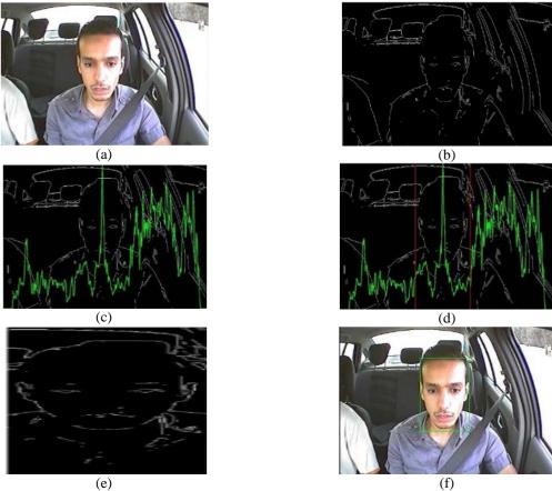
Figure 3: Face detection using symmetry. (a) Original image, (b) Edge detection, (c) Symmetry signal, Localization of the maximum of symmetry, (e) Region of interest ROI (f)Result.
