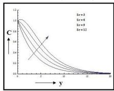
Figure 16: Effects of Soret number on the concentration profiles Ec=0.001, Pr=0.025, M=2, Gr=5, Gm=2, F=3, Sc=0.22, K=1, R=0.30
