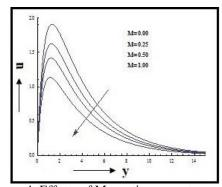
Figure 4: Effects of Magnetic parameter on the velocity profiles Ec=0.001, Pr=0.025, Gr=2, Gm=2, F=3, Sc=0.22, K=1, R=0.30, Sr=3
