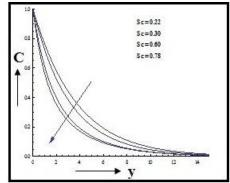
Figure 12: Effects of Schmidt number on the concentration profiles Ec=0.001, Pr=0.025, M=2, Gr=5, Gm=2, K=1, F=3, Sr=3, R=0.30
