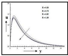
Figure 8: Effects of Chemical reaction parameter on the velocity profiles Ec=0.001, Pr=0.025, M=2, Gr=5,
