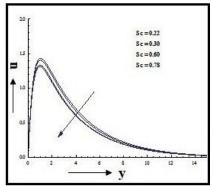
Figure 1: Effects of Schmidt number on the velocity profiles Ec =0.001, Pr=0.025, M=2, Gr=5, Gm=2,
