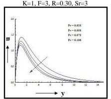
Figure 2: Effects of Prandtl number on the velocity profiles Ec=0.001, Sc=0.22, M=2,Gr=5, Gm=2, K=1, F=3 R=0.30, Sr=3
