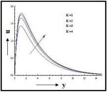
Figure 7: Effects of porosity parameter on the Velocity profiles Ec=0.001, Pr=0.025, M=2, Gr=5, Gm=2, Sc=0.22, F=3, R=0.30, Sr=3
