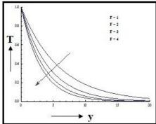
Figure 11: Effects of radiation parameter on the temperature profiles Ec=0.001, Sc=0.60, Pr=0.025, M=0.5, Gr=2, Gm=2, K=1, Sr=3, R=0.30
