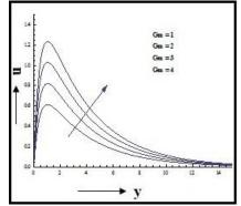
Figure 5: Effects of Modified Grashof number on the velocity profiles Ec=0.001, Pr=0.025, M=2, Gr=2, F=3, Sc=0.22, K=1,R=0.30, Sr=3
