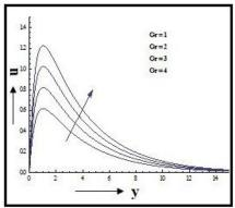
Figure 3: Effects of Grashof number on the velocity profiles Ec=0.001, Pr=0.025, M=2, F=3, Gm=2, Sc=0.22, K=1, R=0.30, Sr=3
