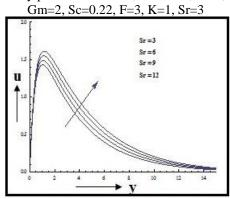
Figure 9: Effects of Soret number on the velocity profiles Ec=0.001, Pr=0.025, M=2, Gr=5, Gm=2, K=1, F=3, Sc=0.22, R=0.30
