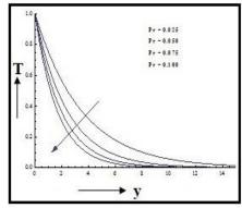
Figure 10: Effects of Prandtl number on the temperature profiles Ec=0.001, Sc=0.22, M=0.5, Gr=2, Gm=2, K=1, F=3, R=0.30, Sr=3
