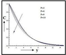
Figure 14: Effects of Radiation parameter on the concentration profiles Ec=0.001, Sc=0.22, Pr=0.025, M=2, Gr=5, Gm=2, K=1, R=0.30, Sr=3
