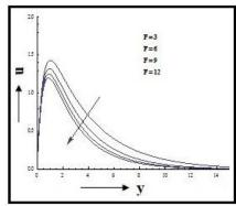
Figure 6: Effects of Radiation parameter on the velocity profiles Ec=0.001, Pr=0.025, M=2, Gr=5, Gm=2, Sc=0.22, K=1, R=0.30, Sr=3
