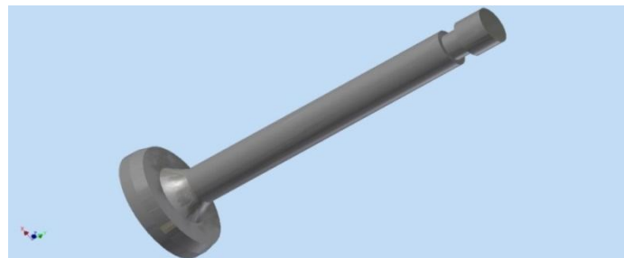
Figure 5: 3D modelling of poppet valve
