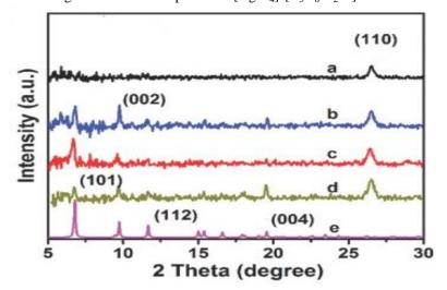
Figure 2: XRD patterns of MOF's nanocomposites
