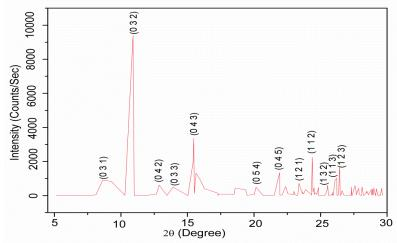
Figure 1: XRD Peak profile of [HgCl<sub>4</sub>]<sup>-</sup> [C<sub>5</sub>H<sub>6</sub> N<sub>2</sub>Cl]<sup>+</sup> MOF.
