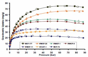
Figure 7: Hydrogen storage in different MOFs. Adsorption data are shown as closed circles, desorption data as open circles.
