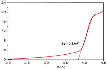
Figure 6: UV-Vis absorption spectra of MOF.
