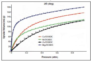
Figure 8: Low-pressure carbon dioxide adsorption for analogs of MOF-74 (Co<sup>II</sup>, Ni<sup>II</sup>, Mg<sup>II</sup>, and Zn<sup>II</sup>).
