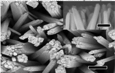
Figure 4: FESEM image of MOF. Scale bars: 200 nm
